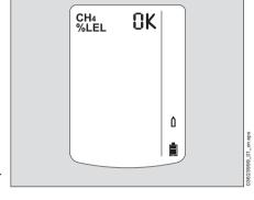
Close the test gas cylinder valve and remove the device from the calibration cradle.
