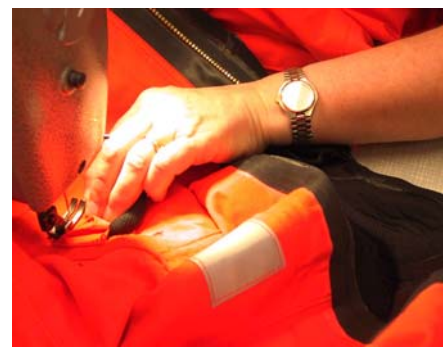
Sew on the pocket so that the stitch at the bottom is covered.
