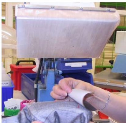
Heat on a patch, reverse the suit, in a cross-over. The patch must cover the stitching from the light pocket.
