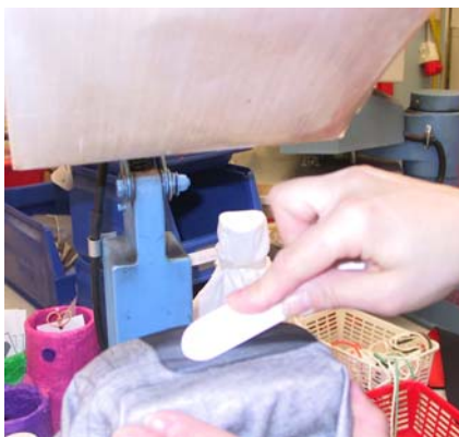
The patch is to be knuckled.
