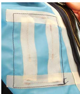
The stitches must be sealed on the reverse side with tape, article no. 1003570 in cross over.
