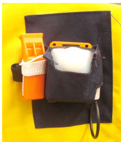
The whistle and new light, article No. 1018938 L6 MCMURDO, MANUALLY is to be mounted.
